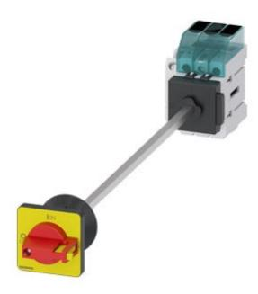
Load disconnector 3LD3, Iu 40 A Main switch 3-pole Rated operating capacity at AC-23 A at 400 V 15.0 kW floor mounting Basic switch with door coupling Central hole mounting 22.5mm Toggle drive red / yellow 48x48 mm with auxiliary switch 10E + 1S
