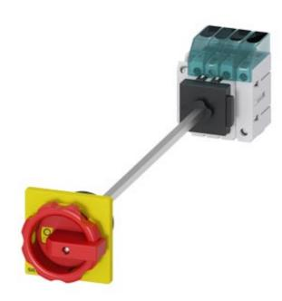
Load disconnector 3LD3, Iu 40 A Main switch 3-pole + N Rated operating capacity at AC-23 A at 400 V 15.0 kW floor mounting Basic switch with door coupling Central hole mounting 22.5mm Rotary actuator red / yellow 66 x 66 mm with auxiliary switch 10E + 1S
