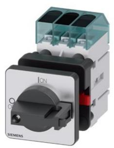
Load disconnector 3LD3, Iu 40 A Main switch 3-pole Rated operating capacity at AC-23 A at 400 V 15.0 kW Front plate mounting Basic switch with Central hole mounting 22.5mm Toggle drive black 48x48 mm
