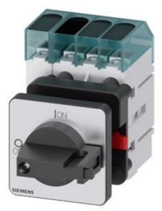
Load disconnector 3LD3, lu 40 A Main switch 3-pole + N Rated operating capacity at AC-23 A at 400 V 15.0 kW Front plate mounting Basic switch with Central hole mounting 22.5mm Toggle drive black 48x48 mm
