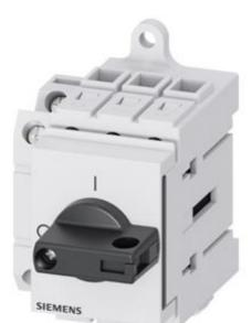
Load disconnector 3LD3, Iu 63 A Main switch 3-pole Rated operating capacity at AC-23 A at 400V 22.0 kW Installation in distribution boards, Basic switch with selector knob black with auxiliary switch 1OE + 1S
