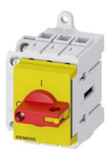
Load disconnector 3LD3, Iu 63 A Main switch 3-pole Rated operating capacity at AC-23 A at 400V 22.0 kW Installation in distribution boards, Basic switch with selector knob red / yellow with auxiliary switch 10E + 1S
