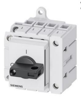
Load disconnector 3LD3, lu 63 A Main switch 3-pole + N Rated operating capacity at AC-23 A at 400V 22.0 kW Installation in distribution boards, Basic switch with selector knob black with auxiliary switch 1OE + 1S
