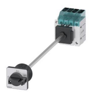
Load disconnector 3LD3, Iu 63 A Main switch 3-pole + N Rated operating capacity at AC-23 A at 400V 22.0 kW floor mounting Basic switch with door coupling Central hole mounting 22.5mm Toggle drive black 48x48 mm with auxiliary switch 1OE + 1S
