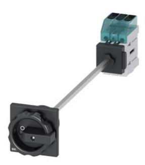
Load disconnector 3LD3, Iu 63 A Main switch 3-pole Rated operating capacity at AC-23 A at 400V 22.0 kW floor mounting Basic switch with door coupling Central hole mounting 22.5mm Rotating drive black 66 x 66 mm
