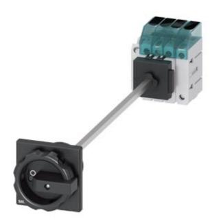
Load disconnector 3LD3, Iu 63 A Main switch 3-pole + N Rated operating capacity at AC-23 A at 400V 22.0 kW floor mounting Basic switch with door coupling Central hole mounting 22.5mm Rotating drive black  $66 \times 66$  mm with auxiliary switch 10E + 1S
