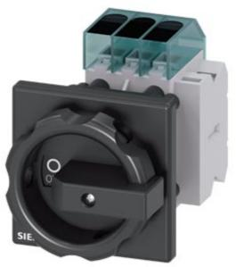
Load disconnector 3LD3, Iu 63 A Main switch 3-pole Rated operating capacity at AC-23 A at 400V 22.0 kW Front plate mounting Basic switch with Central hole mounting 22.5mm Toggle drive black 66x66 mm with auxiliary switch 1OE + 1S
