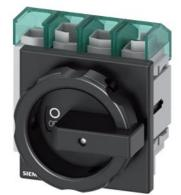
SENTRON, Molded case switch 3LD5 UL, Main switch, 4-pole, certified according to UL489 UL60947-4-1 and IEC60947-3, UL: 60A, SCCR 50kA at 480VAC, Operating power at 480VAC 3-phase: 40hp, IEC: 63A, Operating power at AC-23A at 400V: 30kW, front-mounted, rotary operating mechanism, black, 4-hole mounting of the handle, incl. terminal covers for the infeed side
