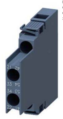
LATERAL AUX.SWITCH BLOCK, SIDE, 1NO+1NC, CURR.PATH: 1NC, 1NO, FOR MOTOR CONTACTORS, SZ S00, SCREW TERMINAL R: 21/22, 33/34 L: 41/42, 53/54
