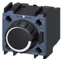
pneumatically time-delayed auxiliary switch, ON-delay, 1-30 s, 1 NO + 1 NC, for mounting to contactors 3RT202
