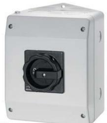
3-P. MAIN CTR. SWITCH IU=16, P/AC-23A AT 400V=7.5KW 1 N-TERMINAL + 1 PE-TERMINAL MOULDED-PLASTIC ENCLOSED, IP65 ROTARY ACTUATOR BLACK
