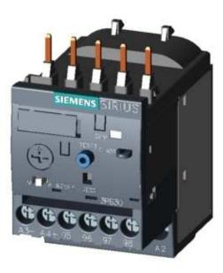
OVERLOAD RELAY 1...4 A FOR MOTOR PROTECTION SIZE S00, CLASS 10 CONTACTOR ASS. MAIN CIRCUIT: SCREW CONN. AUX.CIRCUIT: SCREW CONN. MANUAL-AUTOM.-RESET
