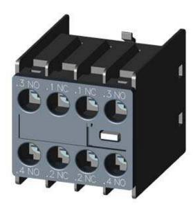
AUX.SWITCH BLOCK,FRONT,2NO+2NC, CURR.PATH: 1NO, 1NC, 1NC, 1NO, F. CONT. RELAYS A. MOTOR CONT., SZ S00 AND S0, SCREW TERMINAL .3 / .4,.1 / .2,.1 / .2,.3 / .4
