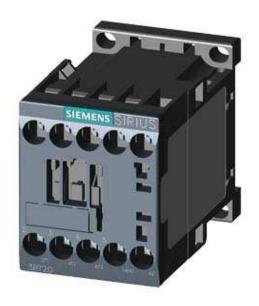
CONTACTOR, AC-3, 3KW/400V, 1NO, AC 230V, 50/60 HZ, 3-POLE, SZ S00 SCREW TERMINAL
