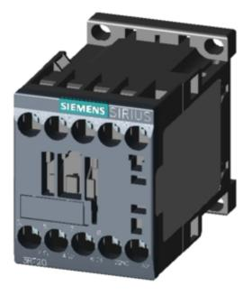
CONTACTOR, AC-3, 5.5KW/400V, 1NC, DC 24V, 3-POLE, SZ S00 SCREW TERMINAL .
