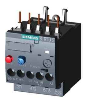
OVERLOAD RELAY 2.2...3.2 A FOR MOTOR PROTECTION SZ S00, CLASS 10, F. MOUNTING ONTO CONTACTOR MAIN CIRCUIT: SCREW TERMINAL AUX. CIRCUIT: SCREW TERMINAL
