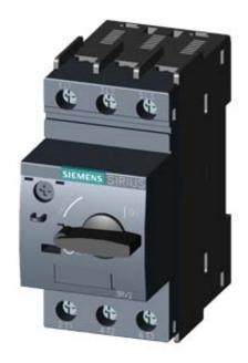
CIRCUIT-BREAKER SZ S00, FOR MOTOR PROTECTION, CLASS 10, A-REL. 0.45...0.63A, N-RELEASE8.2A SCREW CONNECTION, STANDARD SW. CAPACITY
