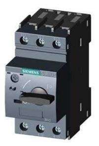
CIRCUIT-BREAKER SZ S00, FOR MOTOR PROTECTION, CLASS 10, A-REL.2.2...3.2A, N-RELEASE 42A, SCREW CONNECTION, STANDARD SW. CAPACITY
