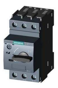
CIRCUIT-BREAKER SZ S00, FOR MOTOR PROTECTION, CLASS 10, A-RELEASE 7...10A, N-RELEASE 130A, SCREW CONNECTION, STANDARD SW. CAPACITY
