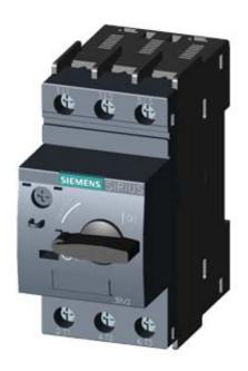
CIRCUIT-BREAKER SZ S0, FOR MOTOR PROTECTION, CLASS 10, A-RELEASE 14...20A, N-RELEASE 260A, SCREW CONNECTION, STANDARD SW. CAPACITY,
