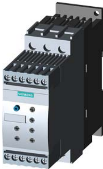
SIRIUS SOFT STARTER, S0, 38A, 18.5KW/400V, 40 DEGR., AC 200-480V, AC/DC 24V, SCREW TERMINALS
