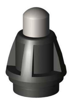
ACTUATOR HEAD FOR POSITION SWITCH 3SE51/52 ROUNDED PLUNGER, FORM B STAINLESS STEEL, WITH 3MM OVERTRAVEL, ACC. TO EN50041
