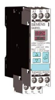
DIGITAL MONITORING RELAY CURRENT MONITORING, 22.5MM FROM 0.05 TO 10A AC/DC OVERSHOOT A. UNDERSHOOT AC/DC 24 TO 240V DC AND AC 50 TO 60 HZ ON AND SPIKE DELAY 0.1 TO 20S HYSTERESIS 0.01 TO 5A 1 CO CONTACT W. OR W/O ERROR MEMORY SCREW CONNECTION REPLACEMENT PRODUCT FOR 3UG3522-1AL20,
