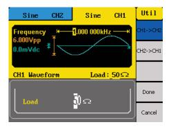
Quickly copy all waveform parameters between channels via the Utility menu. This feature can help you save time when you need to set up two identical output signals.
