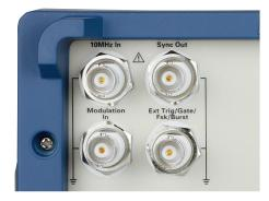
Use the external 10 MHz clock input to synchronize your signals to a master time base. The Sync output generates a TTL pulse for synchronization to a channel's frequency. An external trigger connector is also available for inputting or outputting trigger signals. Dual Channel Function/Arbitrary Waveform Generators 4050 Series
