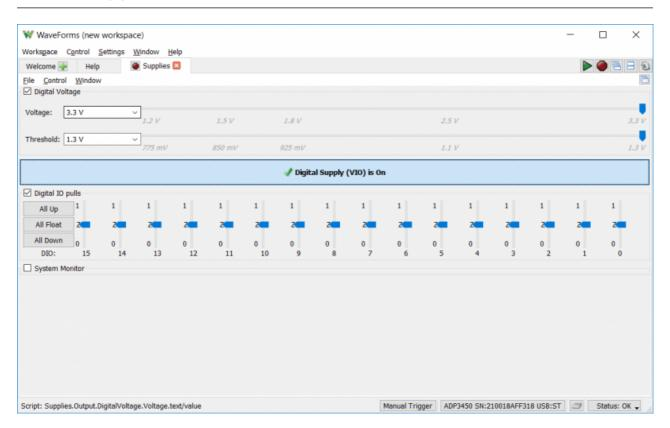
The Analog Discovery Pro (ADP3450/ADP3250) has one programmable Digital Voltage Supply, which can supply between 1.2V and 3.3V, through the Power Supplies ("Supplies") instrument. The Digital I/O Pulls are also configured through the Power Supply instrument, where each digital I/O channel can be individually set to Up, Float or Down.
