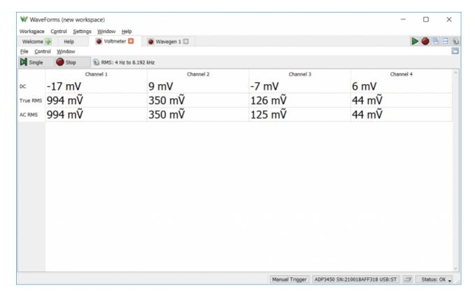
The Analog Discovery Pro (ADP3450/ADP3250)'s analog inputs can be used with WaveForms' Voltmeter instrument to act as a simple 4 channel voltmeter. DC voltages, AC RMS voltages, and True RMS voltages can be viewed for each Scope channel.
