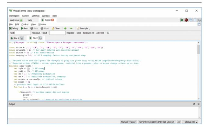
Each of WaveForms' instruments can be controlled through scripts within the WaveForms application itself. WaveForms' "Script" instrument allows the user to write and run JavaScript code that can control the rest of the application through an extensive API (). This allows the user to configure and run many instruments at the same time, in an easily repeatable way.
