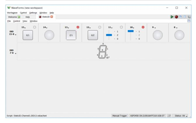
The Analog Discovery Pro (ADP3450/ADP3250) can be used with WaveForms' Static I/O instrument to emulate a variety of user input/output devices on the digital input/output pins. Virtual LEDs, buttons, switches, sliders, and displays can be assigned to specific digital I/O pins, and interacted with within the WaveForms user interface.
