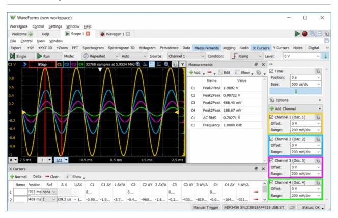
The Analog Discovery Pro (ADP3450/ADP3250) can be used with WaveForms' Oscilloscope instrument to capture analog data via the 4 analog input ("Scope") channels using BNC probes.
