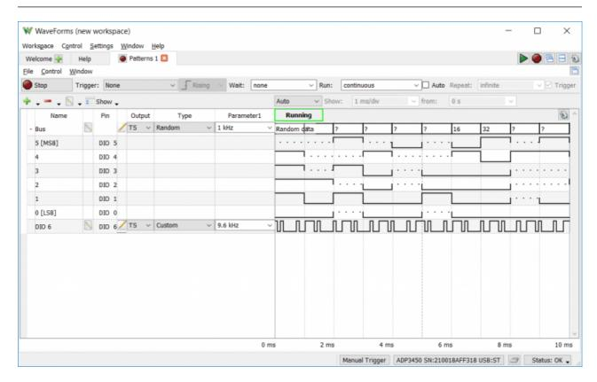
The Analog Discovery Pro (ADP3450/ADP3250) can be used with WaveForms' "Patterns" instrument to generate logic signal sequences on the digital input/output pins. Each channel can be configured to be push/pull, open drain, open source, or three-state logic and set to generate Clock, pulse, random or custom patterns.
