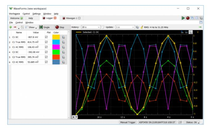
The Analog Discovery Pro (ADP3450/ADP3250) can be used with WaveForms' "Logger" instrument in order to capture large buffers of analog input data on the 4 Scope channels.
