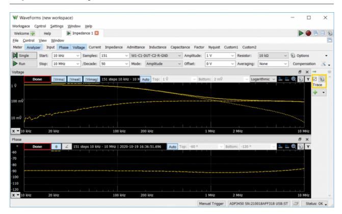
The Analog Discovery Pro (ADP3450/ADP3250) can be used with WaveForms' "Impedance" instrument to view a wide variety of frequency response characteristics of a circuit under test. Input, Phase, Voltage, Current, Impedance, Admittance, Inductance, Factor, and Nyquist plots are all available. In addition, Custom plots can be used to present the results of a wide variety of different mathematical operations on buffered data.
