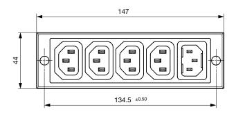
Mounting holes for 3 mm screws
