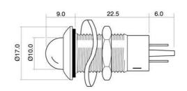
Dimensions in mm (Typical) Not to scale Anode termination indicated by red sleeve Mounting hole to be clean and burr free
