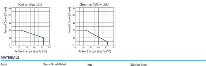
Body Brass, Nickel-Plated Epoxy (LED Lens) Lens Termination (Standard version) I FD Leads Termination (Flying Leads version) Wires, Stripped and Tinned
