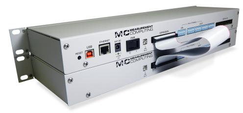
The TC-32 can connect to an Ethernet or USB port. Both the TC-32 and TC-32-EXP include 50-pin connectors that provide access to all DIO channels. Adding the TC-32-EXP expansion device doubles the channel count of the system.
