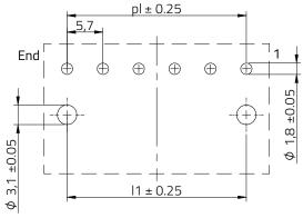
Recommended PCB Layout Thickness : 1.6 mm General Tolerance ± 0.05 mm
