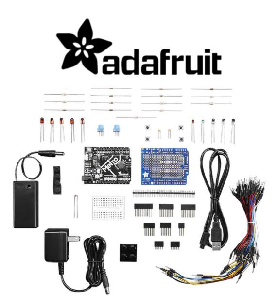
The Adafruit Metro is an ATmega328-based development board. Since it is shaped the same as and Arduino UNO R3, and code/shieldcompatible with it, the Adafruit Metro is easy to use and hacker friendly. This is the perfect beginner kit for learning how to use the Adafruit Metro!
