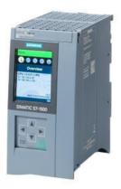
SIMATIC S7-1500T, CPU 1515T-2 PN, central processing unit with 1.5 MB work memory for program and 4.5 MB for data, 1st interface: PROFINET IRT with 2-port switch, 2nd interface: PROFINET RT, 6 ns bit performance, SIMATIC Memory Card required \* \*\*\* approvals and certificates according to entry 109816881 at support.industry.siemens.com to be observed! \*\*\*\*
