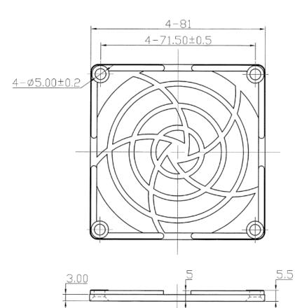
**Material** Plastic - reinforced ABS UL approved Rating UL94V-O
