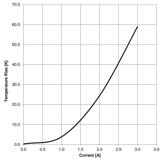
CHECKED GENERAL TOLERANCE PROJECTION METHOD CREATED Würth Elektronik eiSos GmbH & Co. KG EMC & Inductive Solutions KaS CSo DIN ISO 2768-1m Max-Eyth-Str. 1 74638 Waldenburg **WE-WPCC Wireless Power** Tel. +49 (0) 79 42 945 - 0 **Charging Transmitter Coil** ORDER CODE www.we-online.com 760308101104 eiSos@we-online.com DATE (YYYY-MM-DD) BUSINESS UNIT REVISION STATUS PAGE 001.001 Valid 3/6 Ø 20 2017-04-24 WÜRTH ELEKTRONIK
