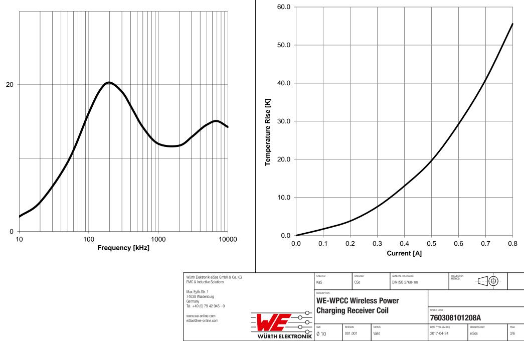
**Typical Temperature Rise vs. Current Characteristics:**
