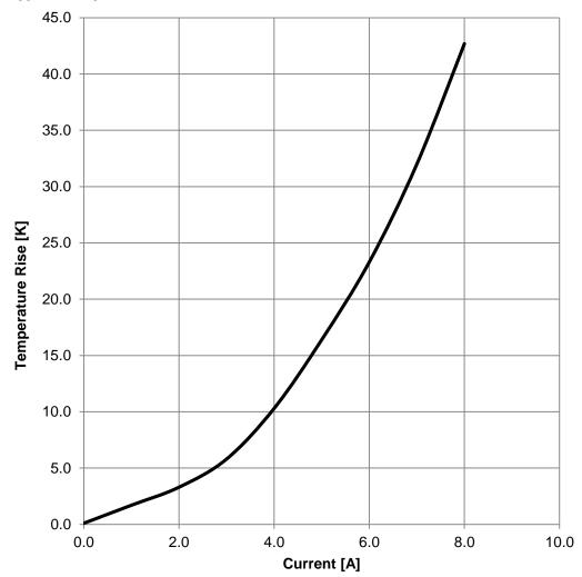
CHECKED GENERAL TOLERANCE PROJECTION METHOD Würth Elektronik eiSos GmbH & Co. KG EMC & Inductive Solutions KaS CSo DIN ISO 2768-1m Max-Eyth-Str. 1 74638 Waldenburg **WE-WPCC Wireless Power** Tel. +49 (0) 79 42 945 - 0 **Transfer Transmitter Coil** ORDER CODE www.we-online.com 760308101304 eiSos@we-online.com DATE (YYYY-MM-DD) BUSINESS UNIT REVISION STATUS PAGE 001.002 Valid 2018-02-01 3/6 WÜRTH ELEKTRONIK
