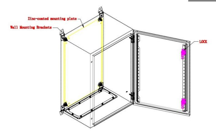
**Application:** A mild steel IP66 industrial wall box suitable for housing electronic and electrical equipment in demanding environments, where the area is prone to frequent hosing or generally wet conditions.
