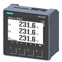
SENTRON PAC3220 LCD 96X96 mm Power Monitoring Device Controll panel instrument for electrical values protocol: Modbus TCP with graphics display U rated input: 690/400V 45-65Hz IE rated input: X/1A oder X/5A AC Power supply: 24 ... 60 V -20/+10 % DC screw connections
