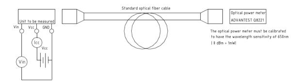
\*3 Pulse response and jitter measuring method
