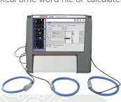
Measurements are done with the voltage input (direct) of the universal board and accessories clamps (standard clamps or flexible clamps)
