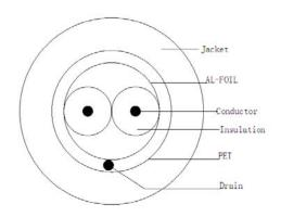
Cable Marking: 1 PAIR 22AWG OVERALL SCREENED DATA CABLE 001M...100M
