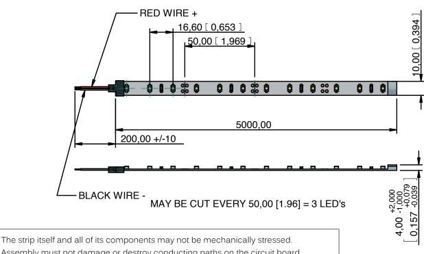
Assembly must not damage or destroy conducting paths on the circuit board.
