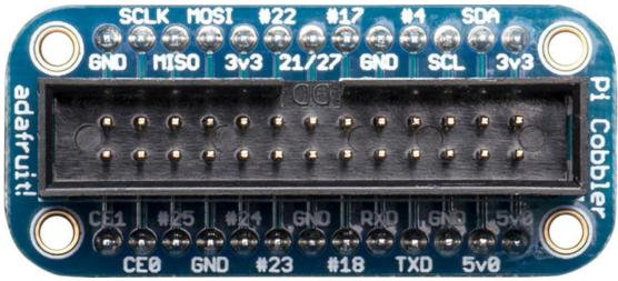
Used to make embedded computer projects on the Raspberry Pi® Model B, the Pi Cobbler from Adafruit, which can break out all the power, GPIO, I2C and SPI pins from the 26 pin header onto a solderless breadboard. This set will make "cobbling together" prototypes with the Pi super easy. Designed for use with Raspberry Pi Model B AND Model A, both revisions. This will not work with the Raspberry Pi 2 or Model A+ or B+.
