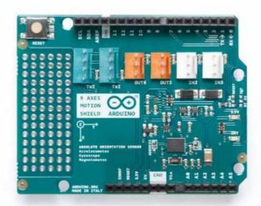
The Arduino 9 Axes Motion Shield is based on the BNO055 absolute orientation sensor from Bosch Sensortec GmbH which integrates a triaxial 14-bit accelerometer, a triaxial 16-bit gyroscope with a range of ±2000 degrees per second and a triaxial geomagnetic sensor with a 32-bit microcontroller running the BSX3.0 FusionLib software.
