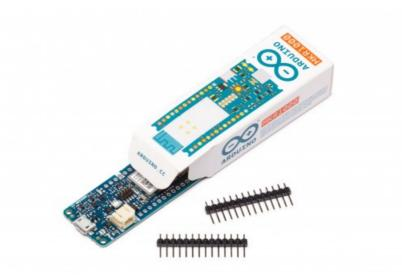
(\*) Note : DO NOT CONNECT to the male JST connector present on the board anything else than a Li-Po battery whose characteristics are compliant with those indicated above. Please DO NOT POWER VIN with more than 5V.
