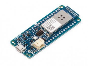
Arduino MKR1000 has been designed to offer a practical and cost effective solution for makers seeking to add Wi-Fi connectivity to their projects with minimal previous experience in networking. It is based on the Atmel ATSAMW25 SoC (System on Chip), that is part of the SmartConnect family of Atmel Wireless devices, specifically designed for IoT projects and devices.
