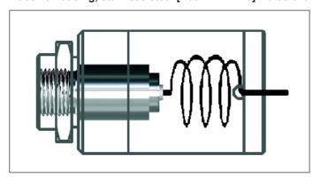
The Massive housing allows reproducible and stable measurements on applications with significant and short-term variation in ambient temperatures. It can be combined with the CF lens [ACCTCFE] or with the protective window [ACCTPWE].
